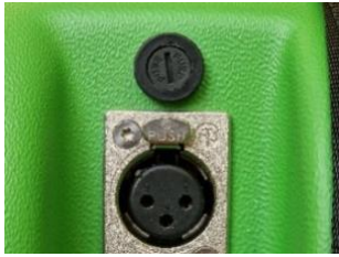
Figure 10: Battery Unit fuse holder (top black circle)
